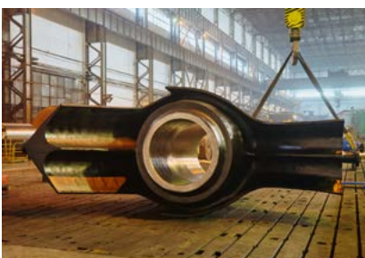
Stern-post casting Part № 21-15206 LK-60
