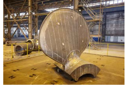
Semi-finished LK-60 right-handed propeller blade
