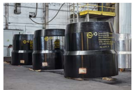
Stern-post weld-in- piece 2-15201 LK-60
